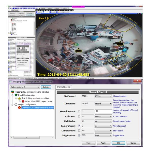
Considering that there is an office with only one entrance, one speed dome and one panorama camera are installed at the center. The speed dome patrols when there's no unusual activity, and focus on the entrance immediately when someone walks through the entrance.
