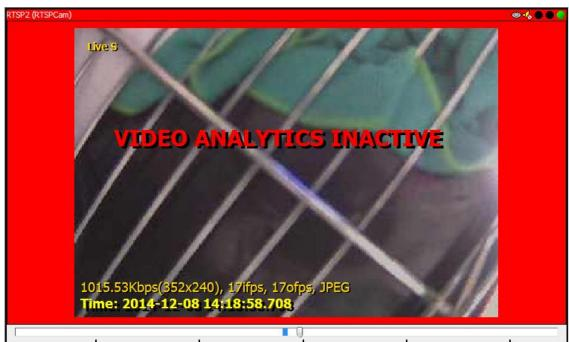
If users setup video analytics but it's not running, NVR fires an alarm of "VIDEO ANALYTICS INACTIVE". There's a problem with this alarm because the state of being inactive is persistent. The alarm will be fired again immediately after users acknowledging it. Users must either enable detection or reset analytics configuration or the alarm can't be dismissed.
